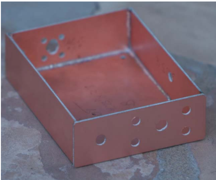
Figure 83. Homebrew case fashioned out of double sided PC board, 5" x 3.5" x 1.375".
