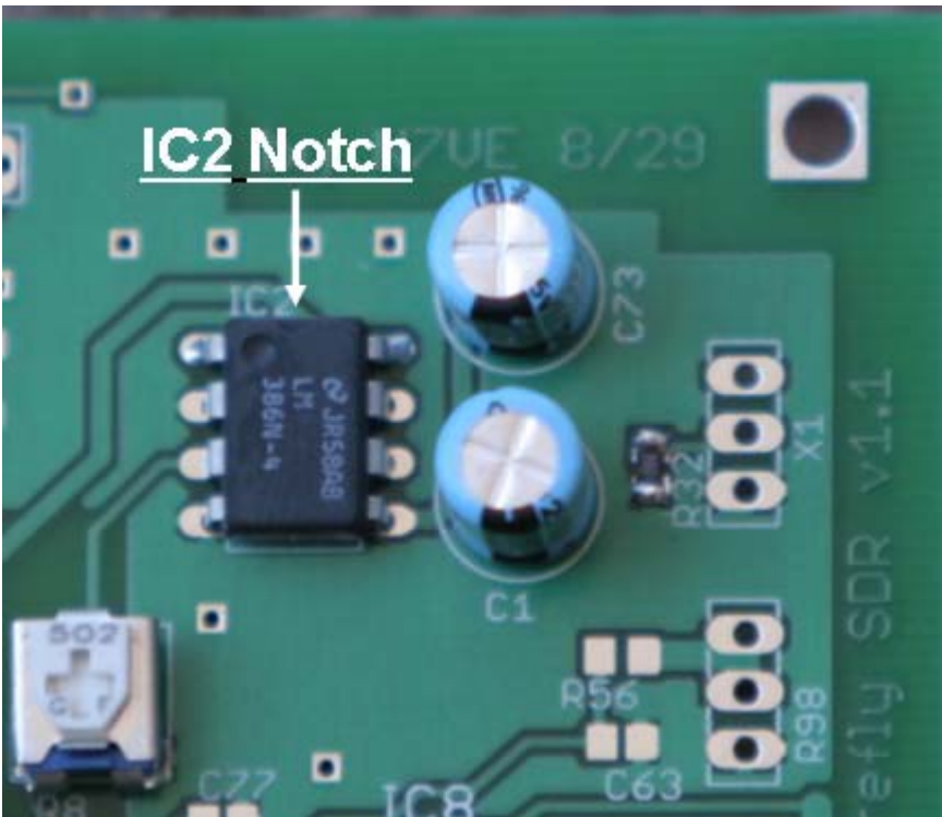
Figure 27. Top side IC2, C73, C1, volume trim pot R8 and R32. Note IC2 polarity and black stripes on C1 and C73.
