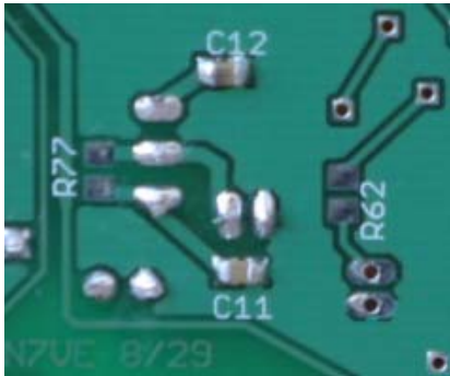
Figure 23. Bottom side of the 6v regulator w/ C11 and C12 installed
