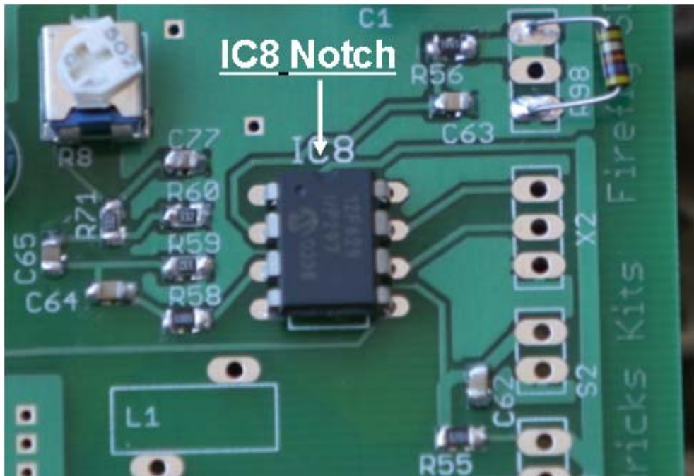
Figure 31. Top side keyer parts. Note the orientation of IC8. IC8 Notch is at the top end.
