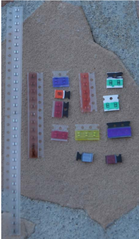
Figure 8. Color coded surface mounted parts. Long clear strip is the 0.1 uf caps (no color code).
